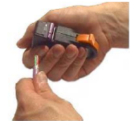
7. The removed insulation remains in the stripper. After releasing the clamp, the remnants can be removed.
