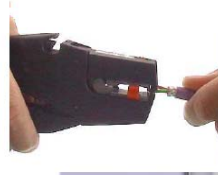
9. After removing the insulation from the cores, the cable can be fitted into the PB connector.
