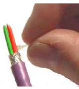
8. Pull the protective foil off the cores.
